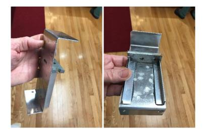
b. I attached the OEM adapter bracket to my custom bracket, then secured my custom bracket to the hitch crossbar using a stainless steel hose clamp routed around the crossbar and through a slot cut in the custom bracket. I then mounted the 7-pole adapter onto the OEM bracket. I used removable (blue) thread-locker on all the bolts.
