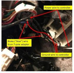
k. I taped up the connections, and zip-tied the wiring up out of the way.
