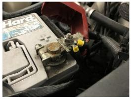
e. I finalized routing the white ground wire from the brake controller to the negative battery post, cut off the excess length, crimped on a ring terminal, then made the final connections to complete the ground side from the brake controller.
