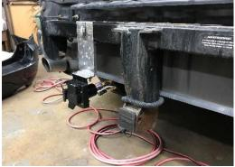
c. I positioned the 7-pole adapter about 6-7 inches to the left of the hitch receiver, then, through a series of careful measurements, incremental cuts, and test fits, I used a utility knife to cut a notch in the lower edge of the rear bumper cover to accommodate the
