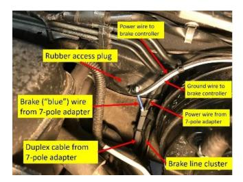
k. I did a final dry-fitting of the duplex cable up and over the brake vacuum booster, then forward alongside the driver's side of the engine bay/inside fender, then to the positive battery terminal, then cut the cable, making sure I had several inches of extra length. I saved the excess length of duplex cable (about 4-5 feet long) for wiring power and ground to the brake controller (see Step 4 below).
