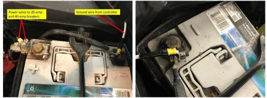
6. Testing connections – I used a <u>tester from Northern Tool</u> to test circuit continuity back to the 7-pole adapter.
