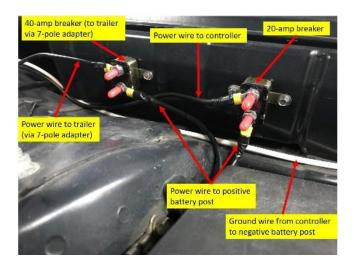
c. I mounted the 20-amp auto-resetting circuit breaker supplied with the ETBC7 kit onto the inside driver's side fender using the kit-supplied self-tapping screws (I had to predrill pilot holes due to limited clearance and angle for the drill).
