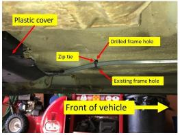
j. I continued to route the duplex cable forward along the inboard face of the driver's side frame rail, attaching the duplex cable at various points using zip ties or <u>rubber-insulated</u> <u>cable clamps</u> purchased from the hardware store. I finished the routing into the engine bay up along the firewall by zip-tying the duplex cable to the brake line group that descends from the brake booster/master cylinder assembly down against the firewall.
