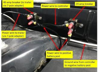
d. I finalized the routing of the black power lead wire from the brake controller to the 20amp breaker, and cut the excess length at the 20-amp breaker. I spliced on a ring terminal and attached the end to the silver post on the circuit breaker. I dry-fit the leftover length to go from the copper terminal of the 20-amp breaker to the positive battery post, then crimped on ring terminals and made the final connections to complete the 12-volt power wire circuit to the brake controller.
