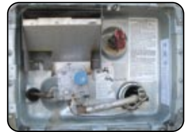
Typical Scamp 6-gallon water heater
