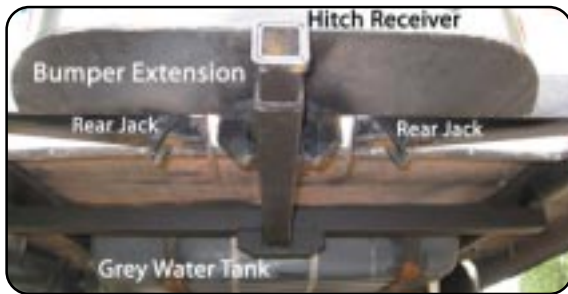
View of underside of the Scamp showing details of the new hitch receiver.
