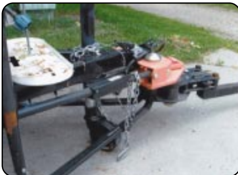
Hensley Arrow anti-sway and load equalization unit.
