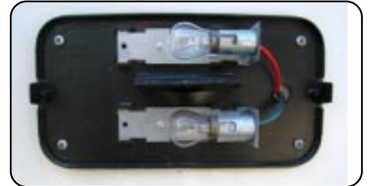
Tail light illustrating the black housing behind the bulbs.
