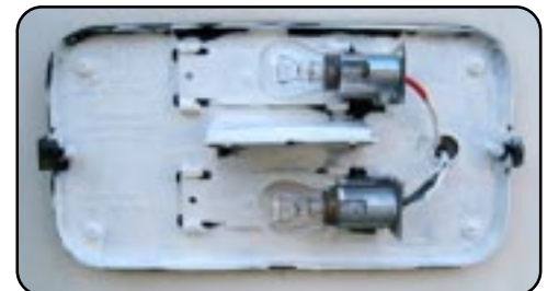
Tail light housing behind the bulbs after painting it white.
