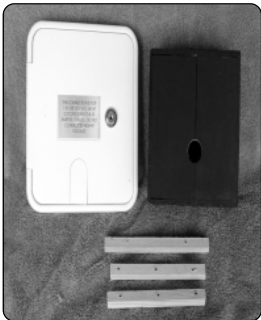
Photo 4 - The hole has been cut, the clearance light moved down and the holes drilled for the mounting screws to secure the housing.
