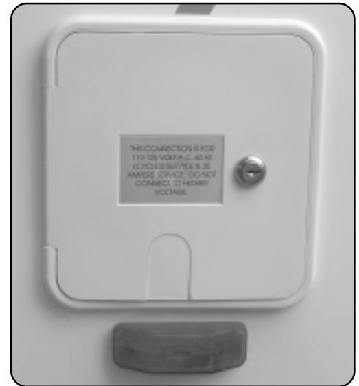
Photo 6 - Finished power cord housing installation and clearance light position.
