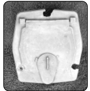
Photo 1 - The original power cord outlet housing with broken flap after removal from Scamp.
