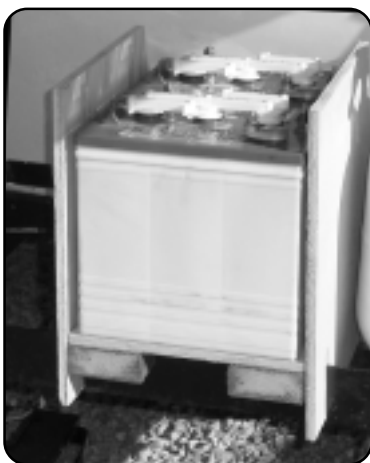
The factory equipped single 12 volt battery was replaced with two 6 volt high amp batteries connected in series. Mounting it between the propane tanks made for a tight fit.
