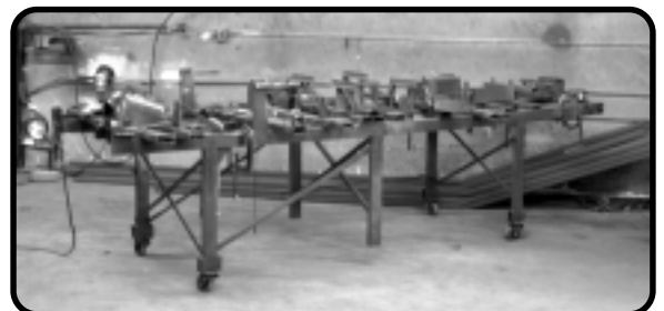
When the Evelands started producing trailers, this jig was designed and built to layout the frames.
