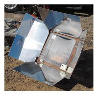
The thermometer inside registered 225 degrees. Just enough to bake the bread without burning it!
