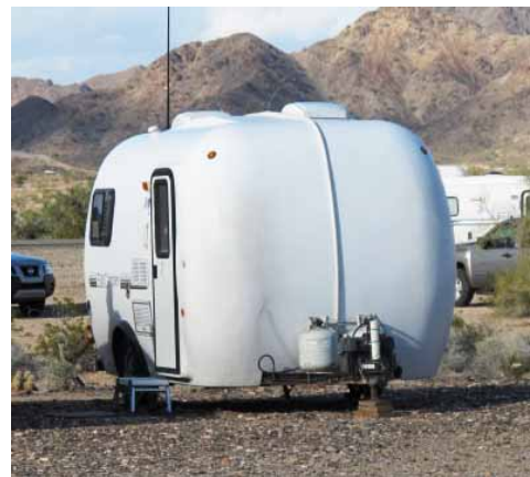
The Egg Camper is unusual in that it is put together different than any other molded fiberglass trailer. Notice all the rest are put together with top and bottom pieces. The Egg Camper is put together with the two halves vertically.
